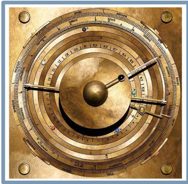
Figure 7. Computer model of the cosmos display. In the centre, the dome of the Earth, the phase of the Moon and its position in the Zodiac;—then rings for Mercury, Venus, true Sun, Mars, Jupiter, Saturn and Date , with “little sphere” markers and smaller markers for oppositions. Scale marks and index letters for the synodic cycles of the planets are inscribed on the planet rings. Surrounding these, the Zodiac and the Egyptian Calendar 2 . The true Sun ring has a “little golden sphere” with “pointer”, as described in the BCI. When the Moon and Sun pointers coincide, the Moon sphere shows black for New Moon; when the pointers are on opposite sides, the Moon sphere shows white for Full Moon 10 . The Head of the Dragon Hand shows the ascending lunar node ; the Tail the descending node . Small triangles on the true Sun ring , near the pointer, show wider and narrower eclipse limits. Eclipses are possible if the Dragon Hand is within these limits. When the Moon pointer is before the Head of the Dragon , the Moon is South of the node; after, it is North of the node—conversely for the descending node. A Date pointer is attached to a narrow date ring, showing the date in the Egyptian calendar 8 .
