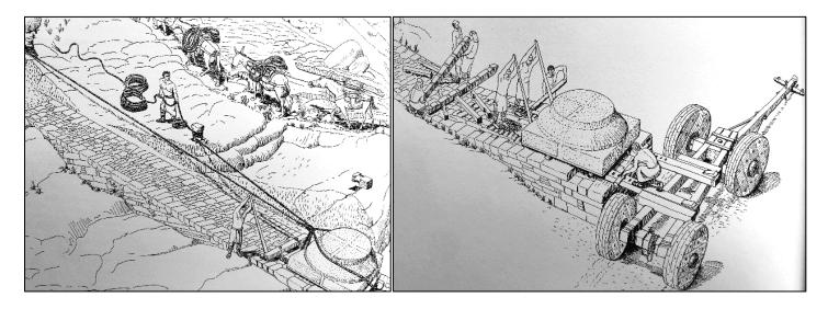
A wooden sled helps move the half-finished capital to a place where it can be safely lifted with ropes and a winch (a lifting device). The block then travels on a stone road down the mountain to a loading platform where it is transferred to a wagon.
