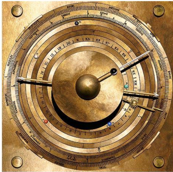
Figure 7. Computer model of the cosmos display. In the centre, the dome of the Earth, the phase of the Moon and its position in the Zodiac—then rings for Mercury, Venus, true Sun, Mars, Jupiter, Saturn and Date , with “little sphere” markers and smaller markers for oppositions. Scale marks and index letters for the synodic cycles of the planets are inscribed on the planet rings. Surrounding these, the Zodiac and the Egyptian Calendar 2 . The true Sun ring has a “little golden sphere” with “pointer”, as described in the BCI: “When the Moon and Sun pointers coincide, the Moon sphere shows black for New Moon; when the pointers are on opposite sides, the Moon sphere shows white for Full Moon 13 ”. The Head of the Dragon Hand shows the ascending lunar node; the Tail the descending node. Small triangles on the true Sun ring, near the pointer, show wider and narrower eclipse limits. Eclipses are possible if the Dragon Hand is within these limits. When the Moon pointer is before the Head of the Dragon, the Moon is South of the nodes; after, it is North of the node—conversely for the descending node. A Date pointer is attached to a narrow date ring, showing the date in the Egyptian calendar 2 .
